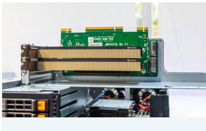
Supermicro SYS E403 14B FRN2T With Two NVIDIA L4 GPUs In Risers
