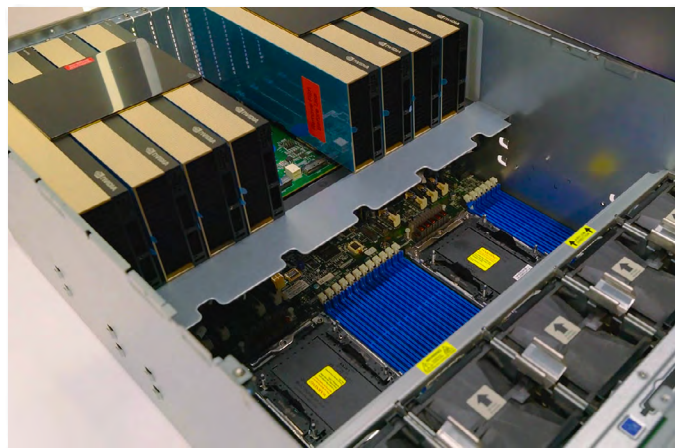
Supermicro SYS-522GA-NRT with 8x NVIDIA H200 NVL and NVLink Bridges
