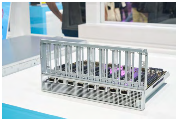
Supermicro NVIDIA MGX PCIe Switch Board With NVIDIA ConnectX 8 SuperNICs For 8x PCIe GPU Servers NIC Ports Large
