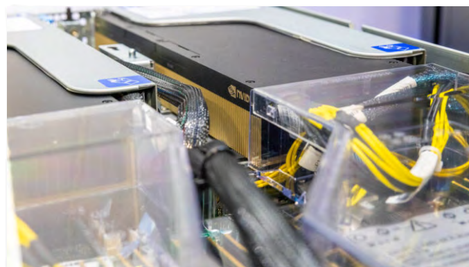
Supermicro SYS 212GB NR Server With Airflow Routing To NVIDIA H100 NVL
